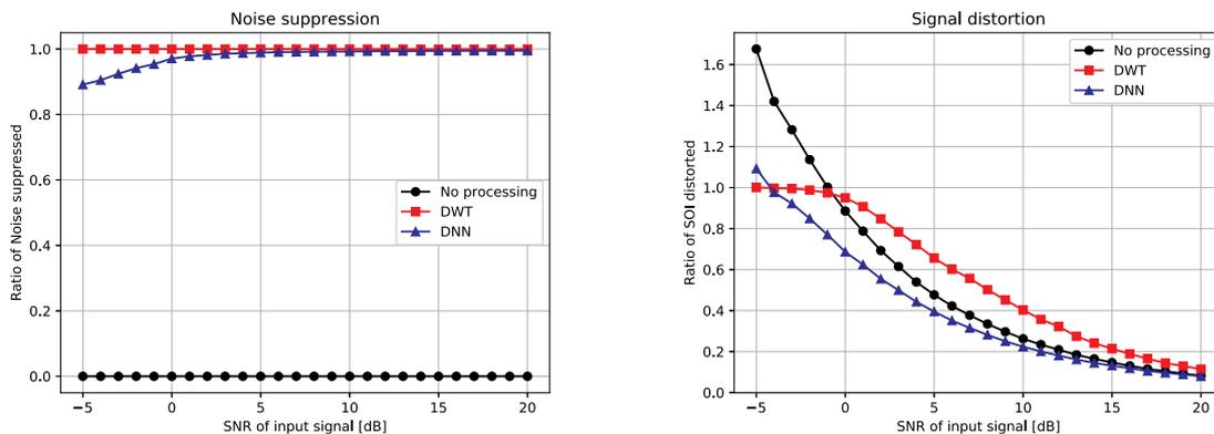
Abbildung 5: Results for noise suppression and distortion introduced by DWT and ML-based denoising algorithms
