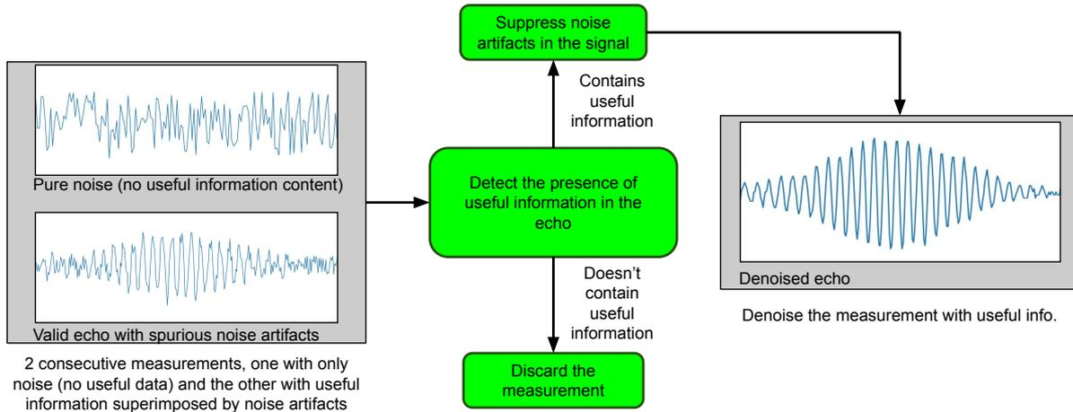
Abbildung 1: The 2-step machine learning based approach of filtering the noise signals with no actual content and further process the valid echoes to suppress spurious noise artifacts
