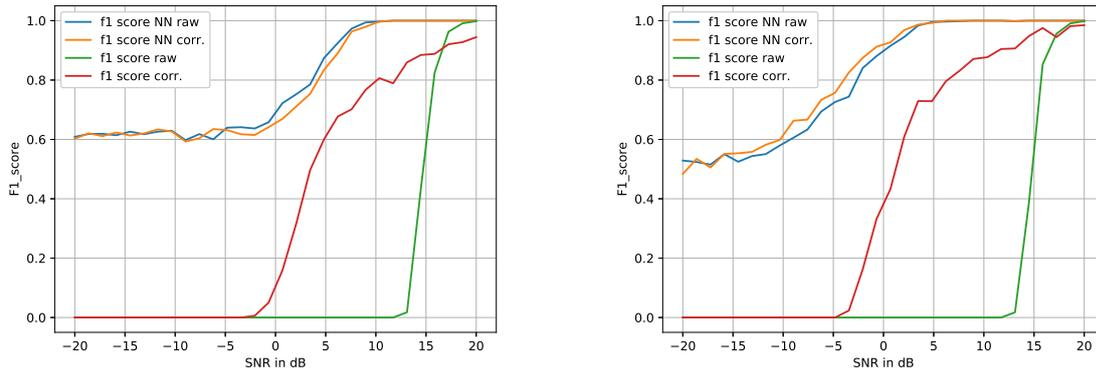
Abbildung 4: Results for echo/noise classification on gravel (ANN trained only for smooth terrain) and mixed terrain types
