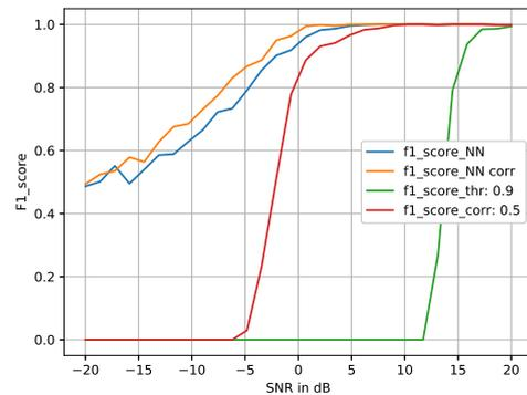
Abbildung 3: Results for echo/noise classification on smooth terrain
