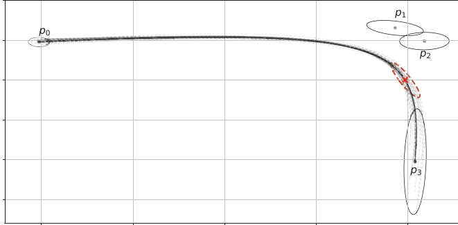
Figure 2: Example of a trajectory representation with n = 3, d = 2 . The solid line corresponds to the mean trajectory and the dashed lines are samples from the density. Parameters, i.e. control points, are indicated at the mean values and with 95% confidence intervals. The red dashed ellipse encloses a 95% confidence region for the position of the object at \tau = 0.7 .
