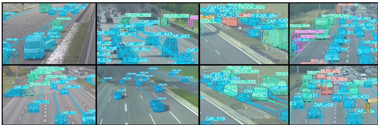
Figure 1: Our dataset provides a visual representation of highway accidents with 3D box annotations, track IDs, instance masks, and vehicle trajectories. The accidents were captured using roadside cameras on the A9 Test Bed for Autonomous Driving. The scenes include crashes, overturned vehicles, and some instances of cars catching fire.
