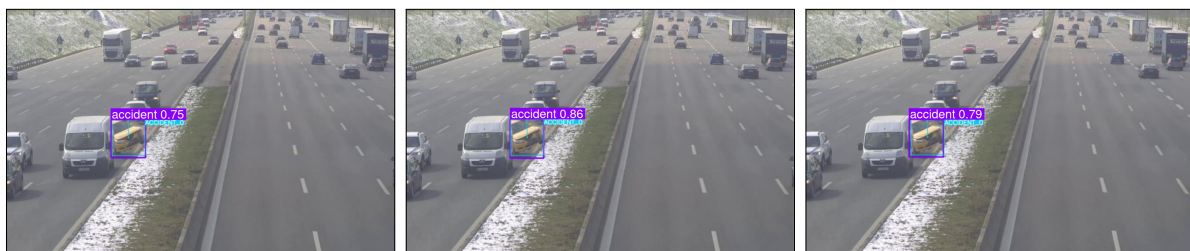
Figure 2: Visual comparison of the accident detection results (purple) on the test set of our accident dataset. Labeled accidents are displayed in turquoise. This test sequence shows a car accident scenario with a yellow car and a white van. We train object detection models with different input image resolutions (1920 px, 1280 px, and 960 px) and find out that an image resolution of 1280 px works best.
