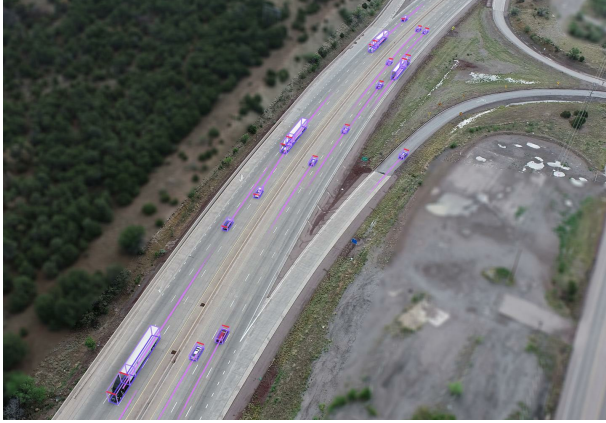
Figure 2: Drone recording annotated with 3D bounding boxes from DeepScenario
