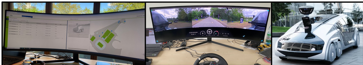
Figure 1: Dispatcher HMI (left, copyright 2024 EDAG Group) and remote operator HMI (middle, copyright 2024 T-Systems) for the operation center of the CityBot (right, copyright 2023 EDAG Group)
