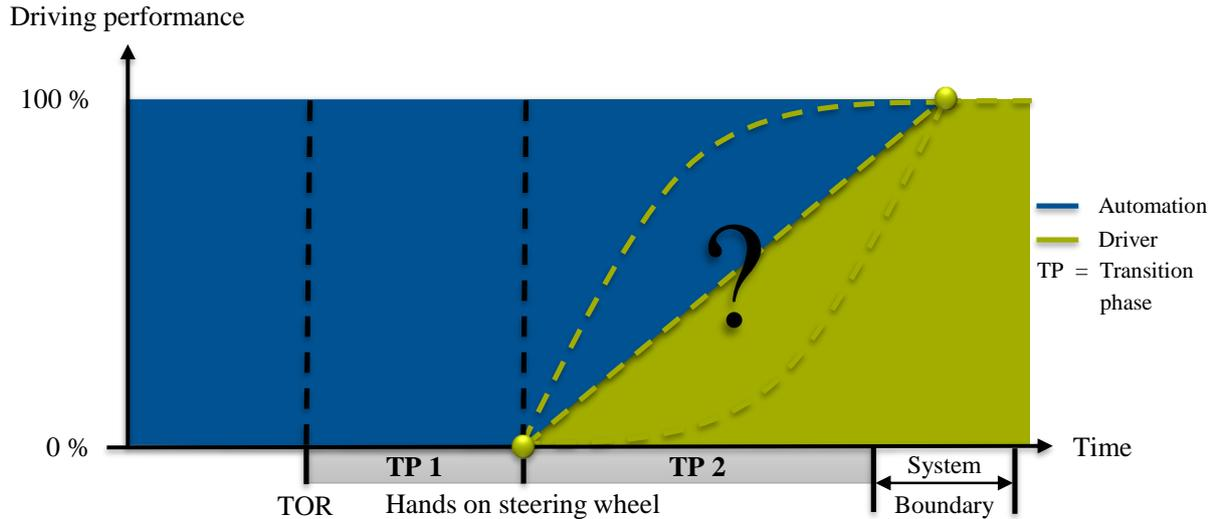
Figure 4: New approach applied on the schematic course of the driving performance during the transition process
