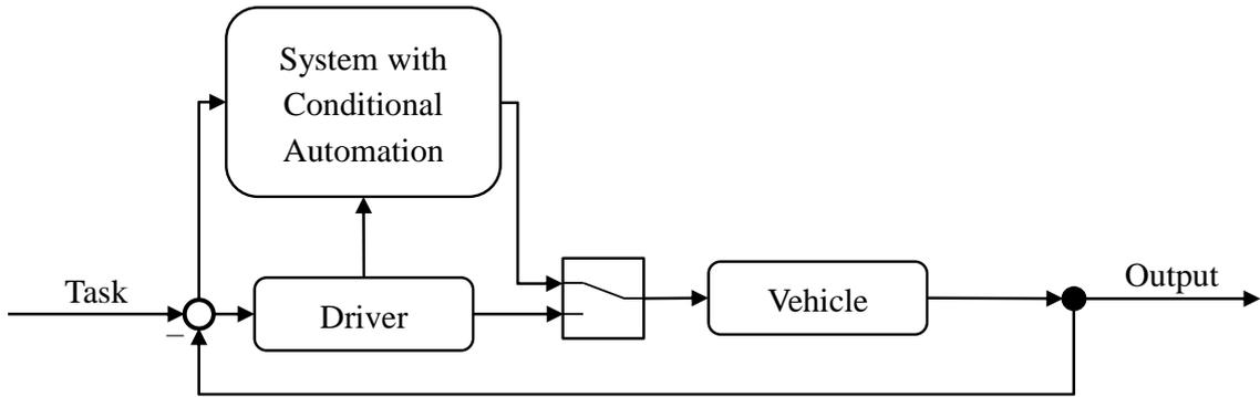
Figure 2: Block diagram of a drive with assistance systems. Adapted from Kienle [14]
