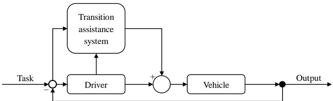
Figure 3: Block diagram of the cooperative transition phase
